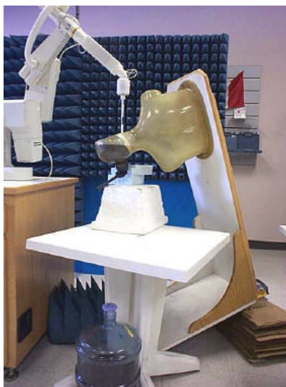
Figure 6.1. IDX system with tilted “conventional phantom and Globalstar phone with antenna tilted-right
