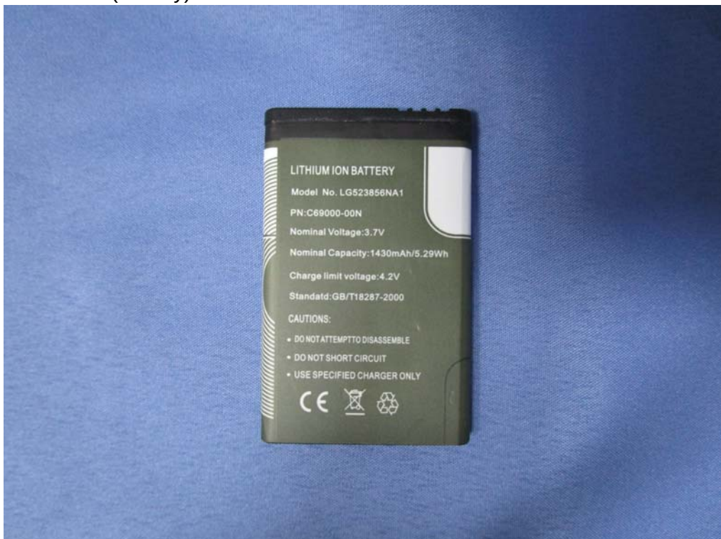
(20) EUT Photo (Battery)
