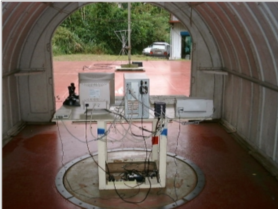
Radiated Emission Setup Photos (Worst Emission Position)
