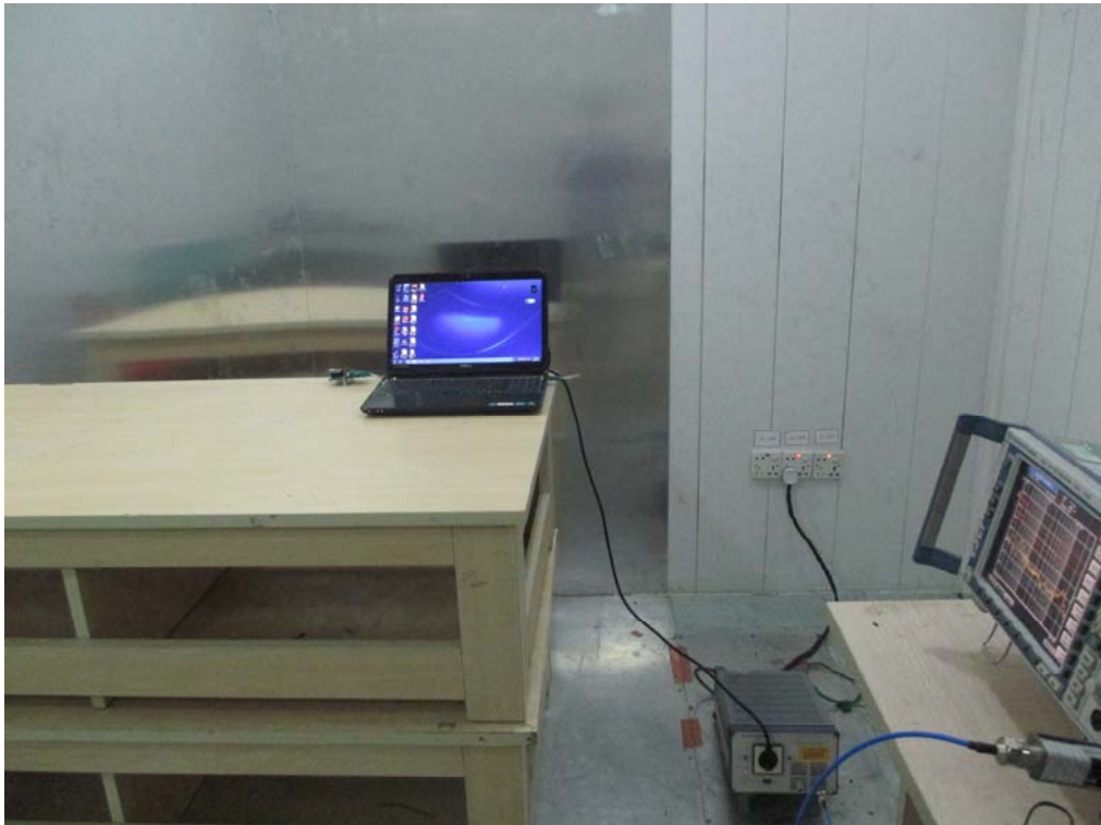
FCC RADIATED EMISSION TEST SETUP
