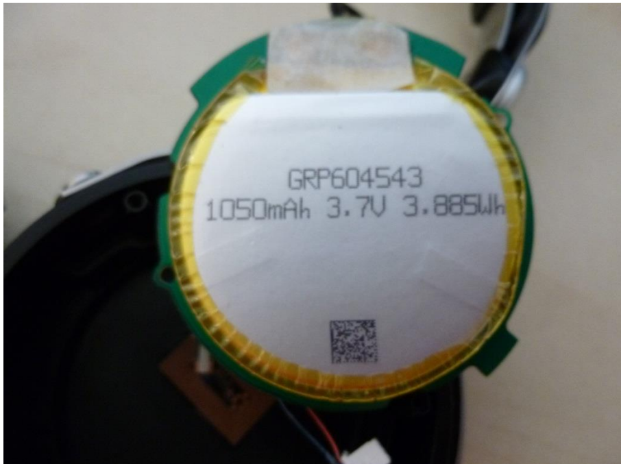
Photo 10: PCB 1 back side view (battery pack)
