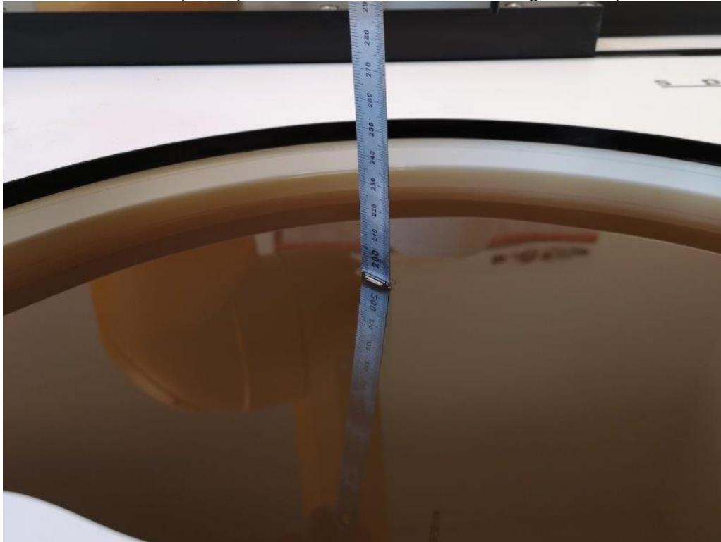
Photo 1: Liquid depth HBBL600-10000MHz Simulating Head Liquid
