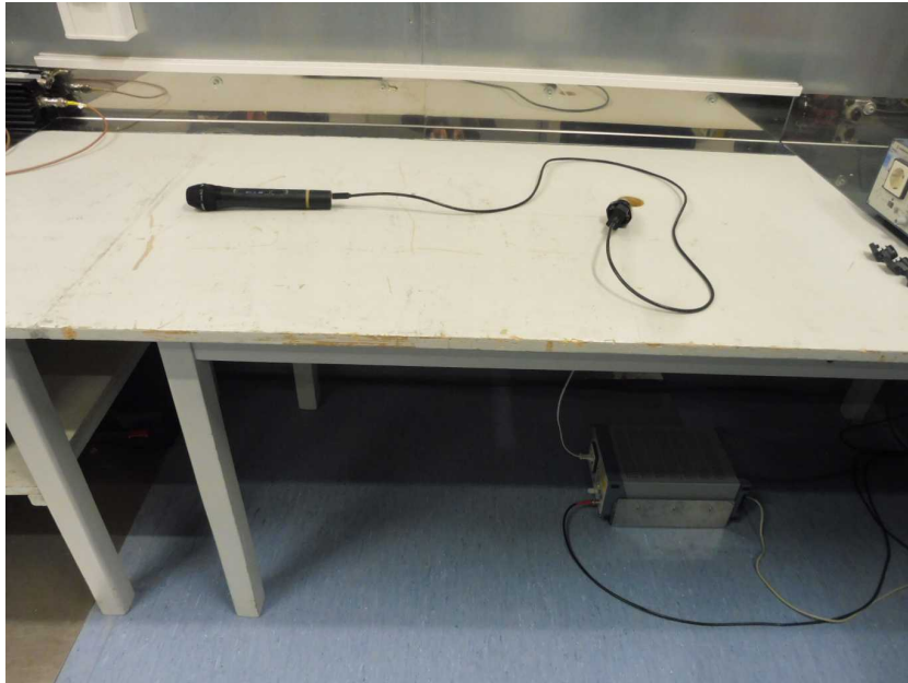
Photo 9: AC conducted emission test setup
