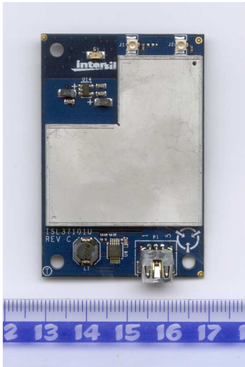
ISL37101U PCB front with shield
