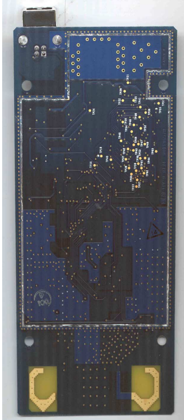
ISL37300XU PCB Rear view without shields (RF)
