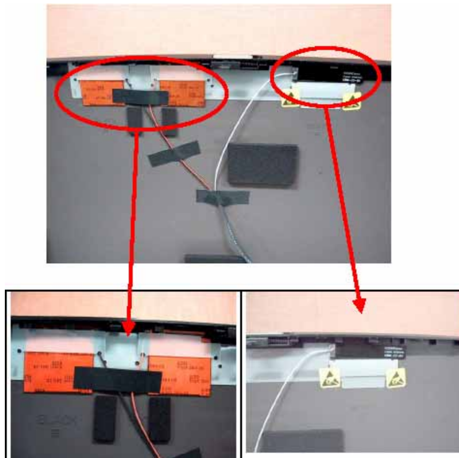
< 2.4 GHz* and 5 GHz WLAN antenna assemblies >
