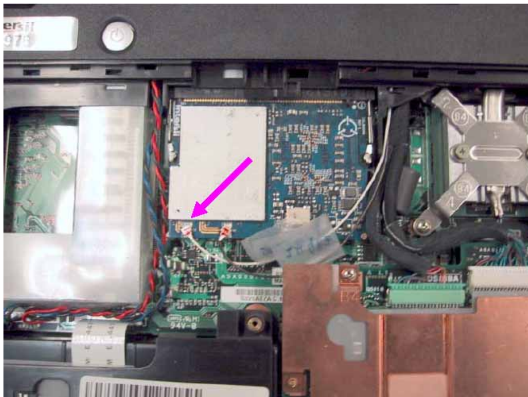
< D.U.T. installed in the miniPCI slot – Close-up view >
