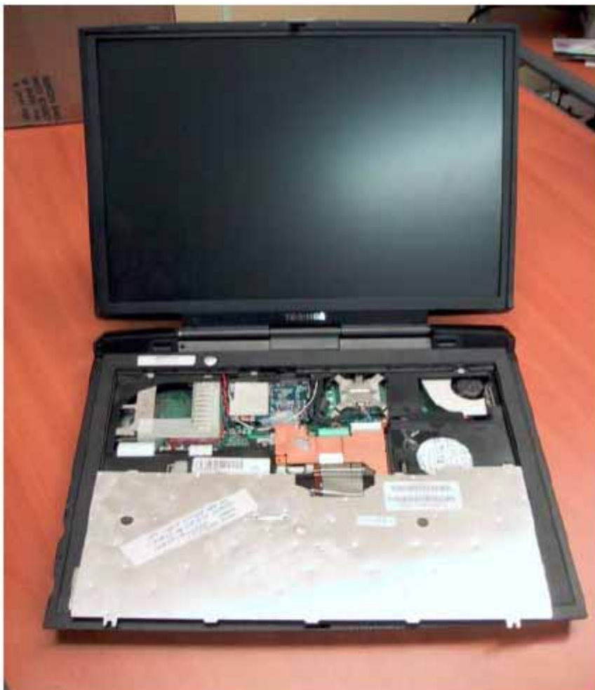
< D.U.T. installed in the miniPCI slot >
