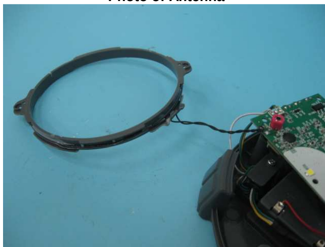
Photo of Antenna
