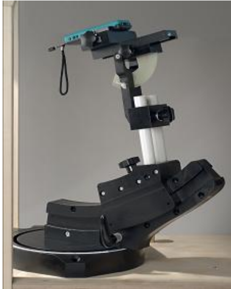
F-2. Device Holder for Transmitters
