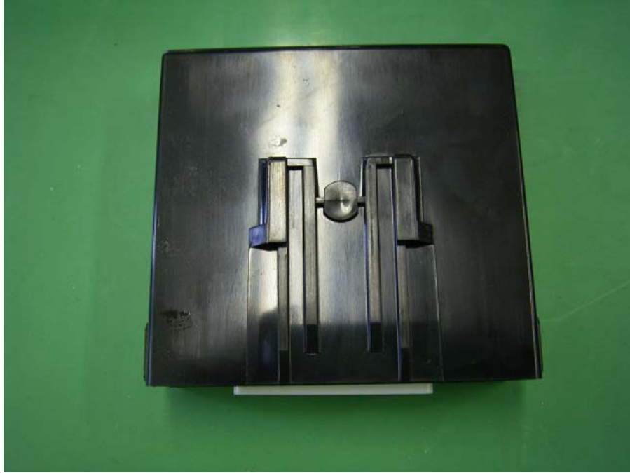
Figure 8.2 G8D—640M—ECU appearance (back view)
