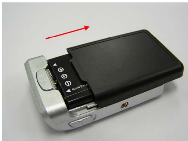
Figure 2 Open the cover of battery
