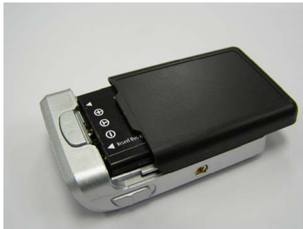
Figure 5 Slide the cover of battery to close
