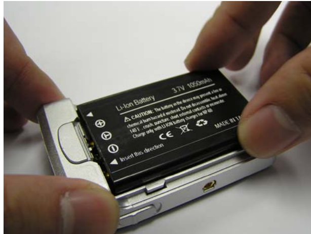
Figure 4 Fit new battery into i-Blue
