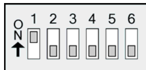
Figure B.8. RS-232 DIP Switch Settings
