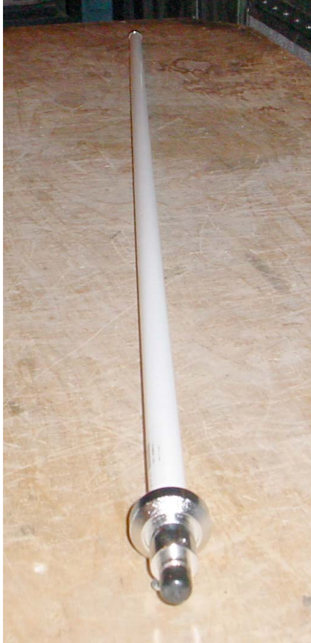
D-Link Antenna (P/N: A24-F15NF; Max. Antenna Gain = 15 dBi)
