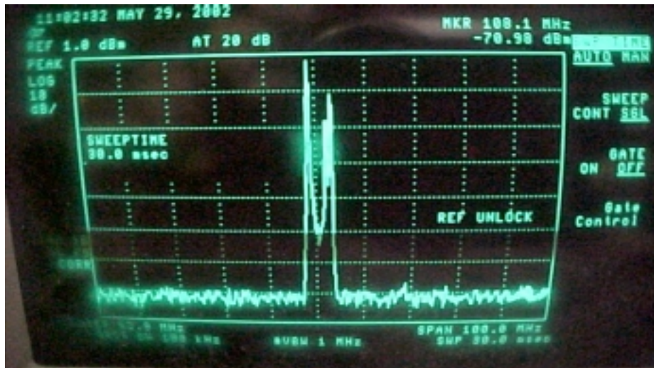
Figure 4-9. Products Above the 70-dB Noise Floor of the Spectrum Analyzer (1 of 2)
