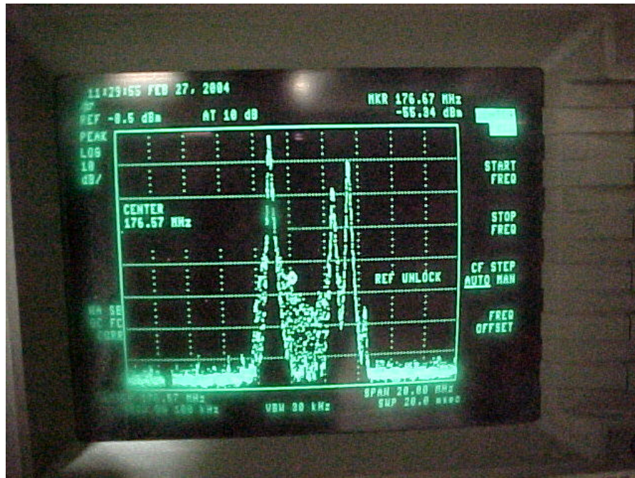
Figure 4-10. Products Above the 70-dB Noise Floor of the Spectrum Analyzer (2 of 2)
