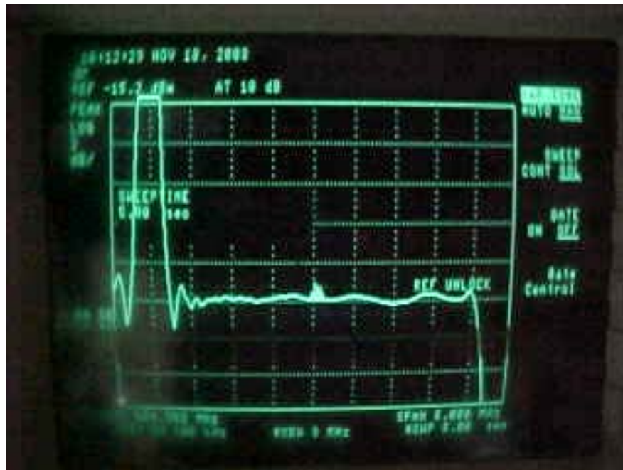
Figure 4-3. Graph of Detected Video Frequency Response
