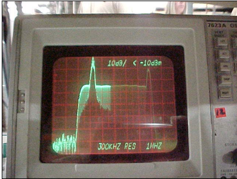
Figure 4-7. Channel Occupied Bandwidth
