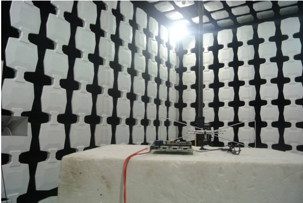
ERP Test, Radiated Spurious Measurement(30MHz to 1GHz) Setup
