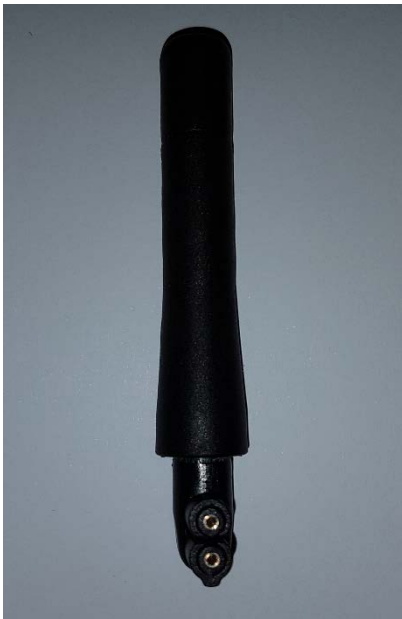
Helix Antenna with unik Kamstrup connector.
