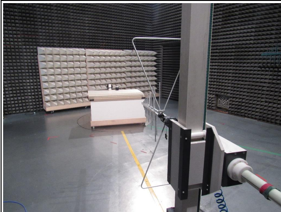
Setup for measurements below 1 GHz (Pit Antenna)
