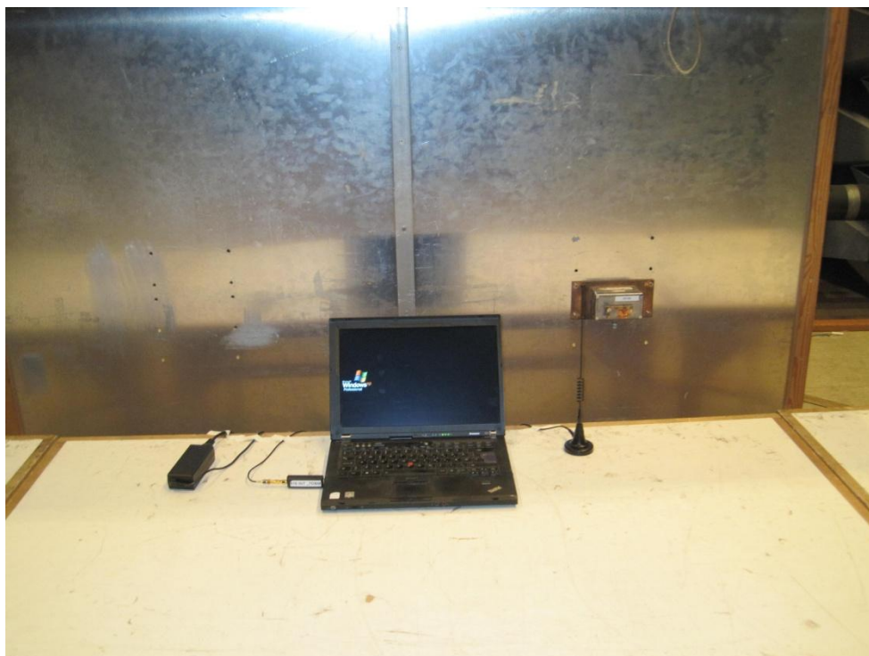
Photo 4.2.1 Test setup regarding measurement of radio conducted limits, AC Mains.
