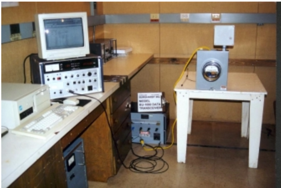
PHOTOGRAPH 3 VIEW OF BU-1000 AND SUPPORT EQUIPMENT: (MRU Board, Meter Dial Encoder, Enclosure and 173 MHz Dipole)
