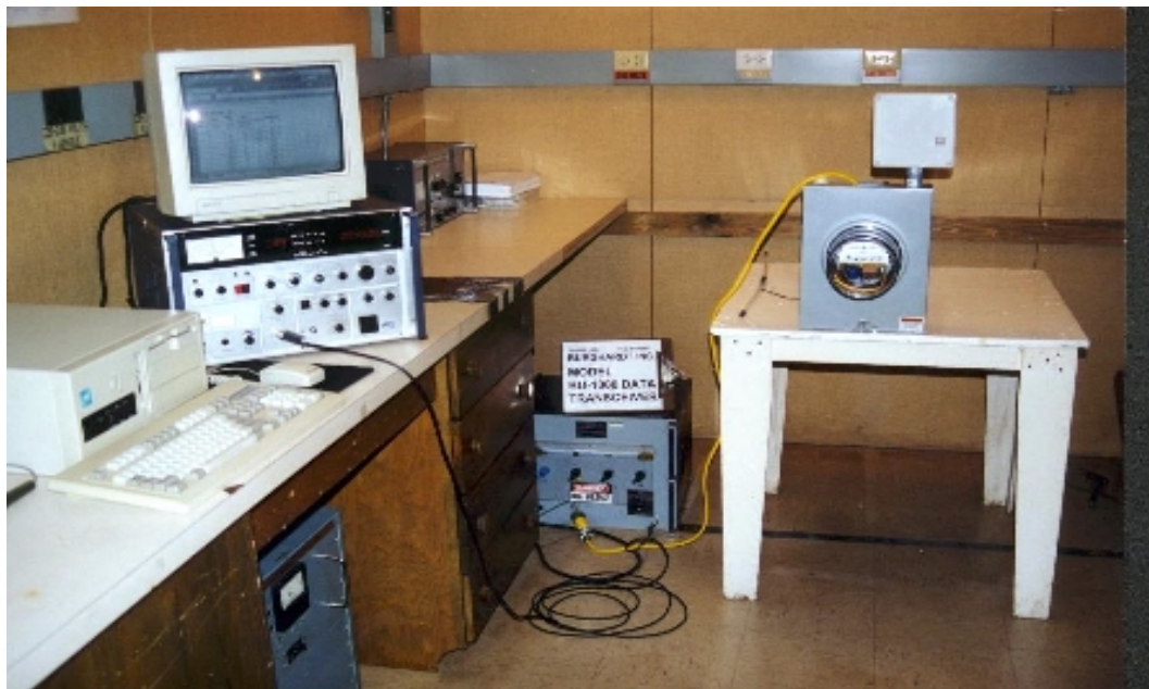
PHOTOGRAPH 4 TERMINAL DISTURBANCE VOLTAGE EMISSIONS CONNECTION TO MEASUREMENT SET
