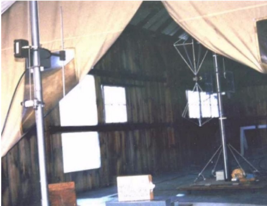
PHOTOGRAPH 7 RADIATED ELECTRIC FIELD EMISSIONS TESTS: SUBSTITUTION MEASUREMENTS
