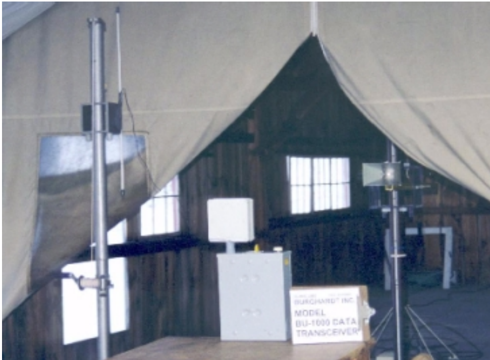
PHOTOGRAPH 9 RADIATED ELECTRIC FIELD EMISSIONS TESTS: 1 TO 5 GHz MEASUREMENTS
