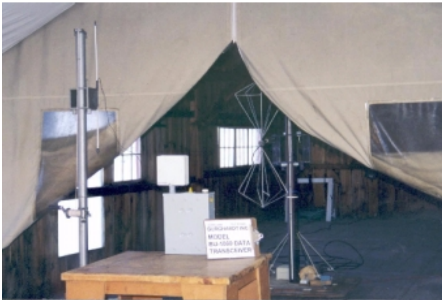
PHOTOGRAPH 6 RADIATED ELECTRIC FIELD EMISSIONS TESTS: 30 TO 300 MHz MEASUREMENTS
