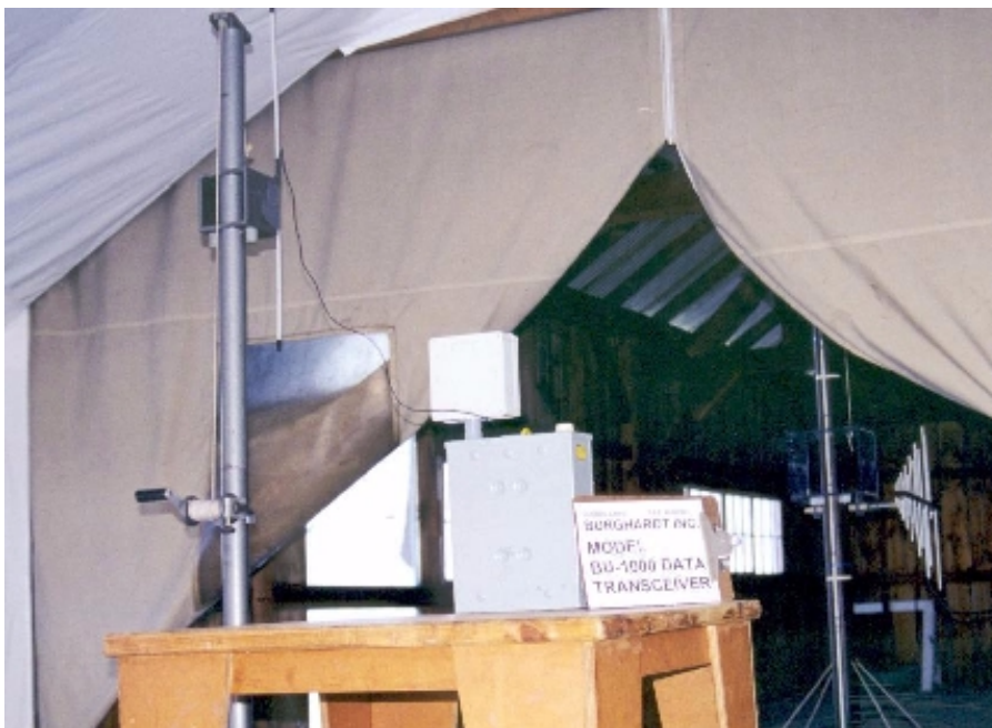
PHOTOGRAPH 8 RADIATED ELECTRIC FIELD EMISSIONS TESTS: 300 TO 1000 MHz MEASUREMENTS
