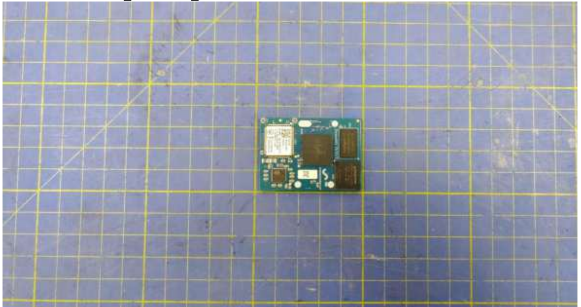
IMG_20250327_093634 S1955 StreamUnlimited Wi-Fi Module
