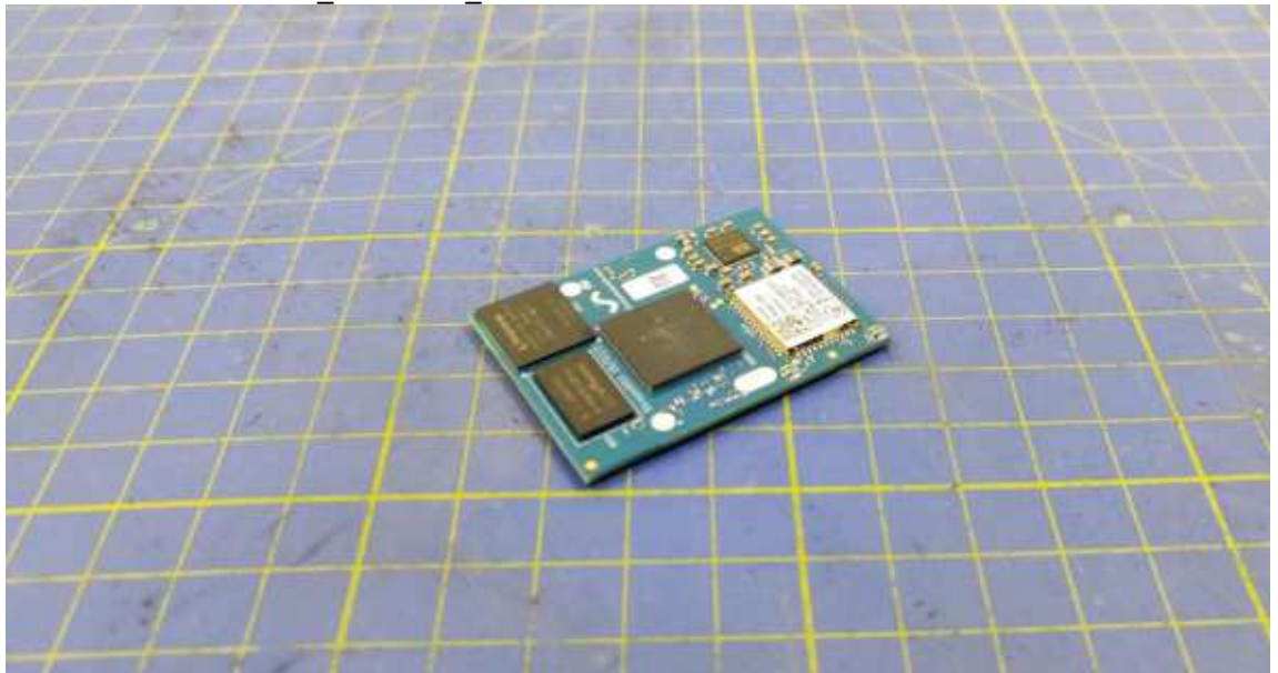
IMG_20250327_093652 StreamUnlimited Wi-Fi Module
