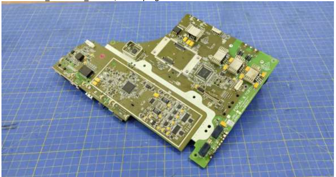
IMG_20250327_101110, Primary Digital PCB – Ethernet shield cover removed
