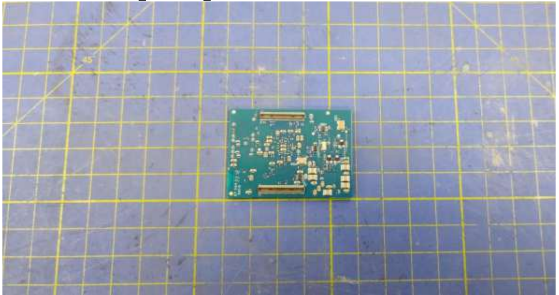
IMG_20250327_093708 StreamUnlimited Wi-Fi Module
