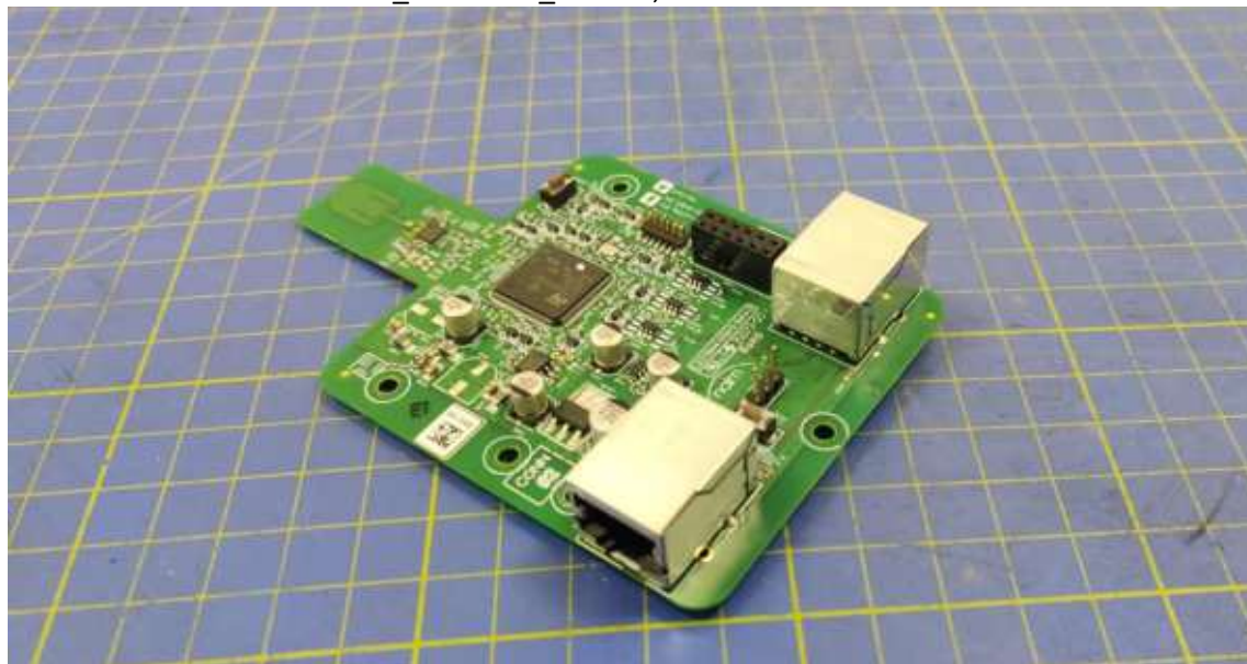
IMG_20250327_104647, UWB Antenna PCB
