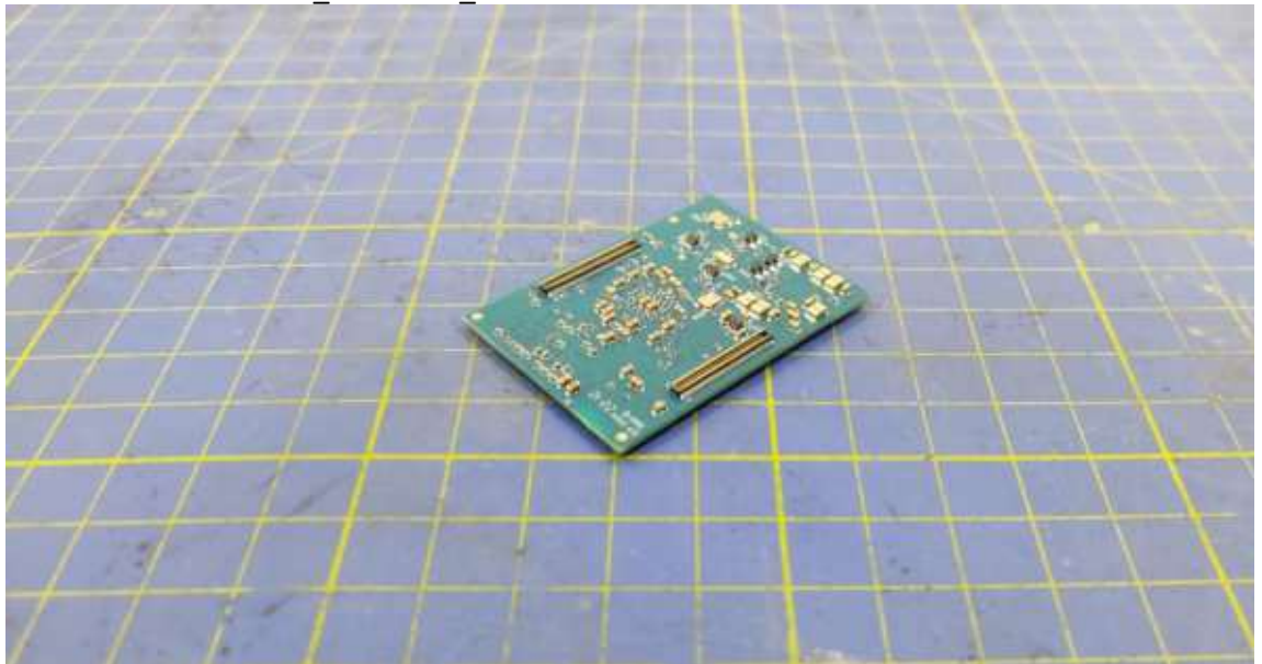
IMG_20250327_093716 StreamUnlimited Wi-Fi Module
