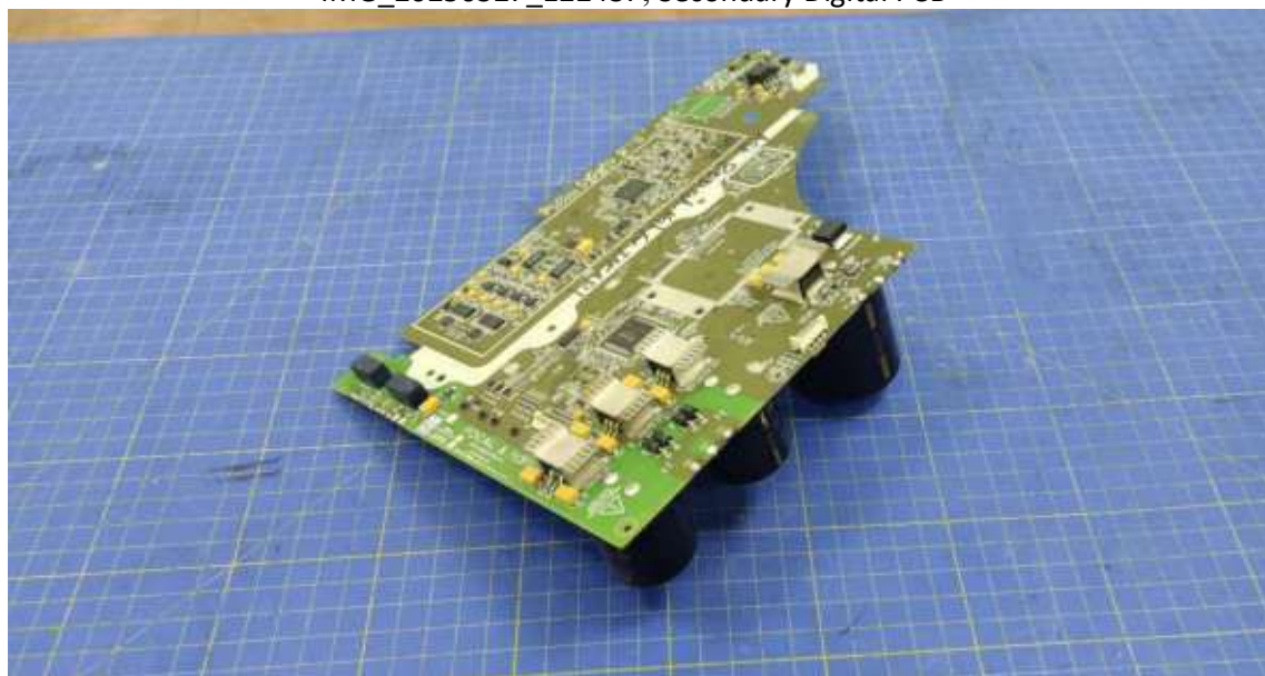
IMG_20250327_122437, Secondary Digital PCB
