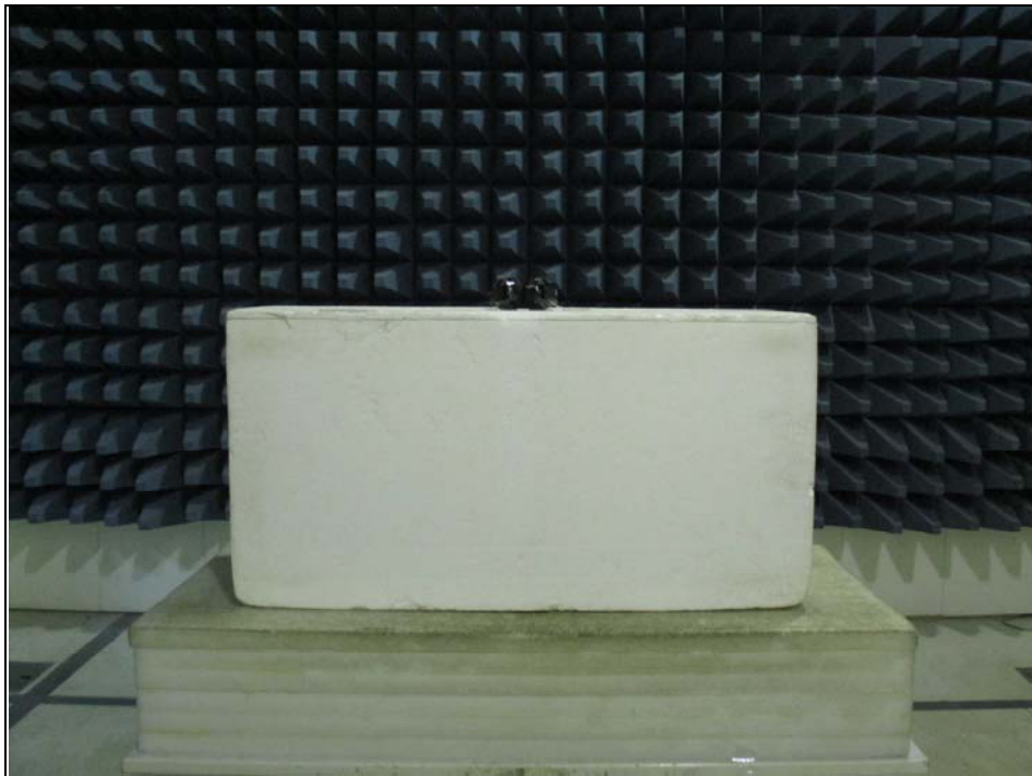
Radiated Emission Test above 1GHz
