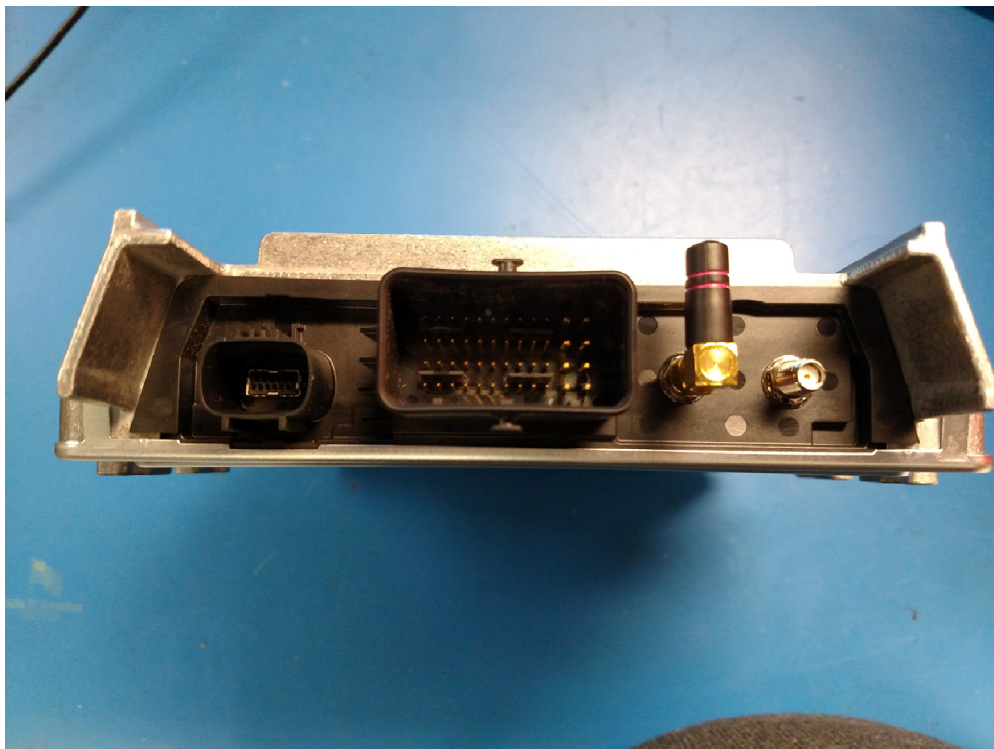
End View SMA WiFi Connectors, Stubby Antenna, Main Connector, Ethernet Connector
