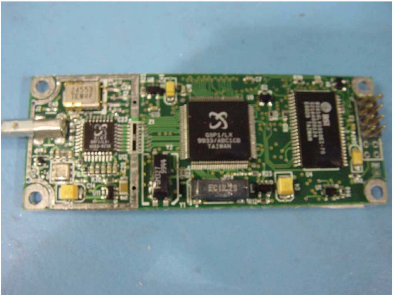
GPS module with RF shield removed (bottom)
