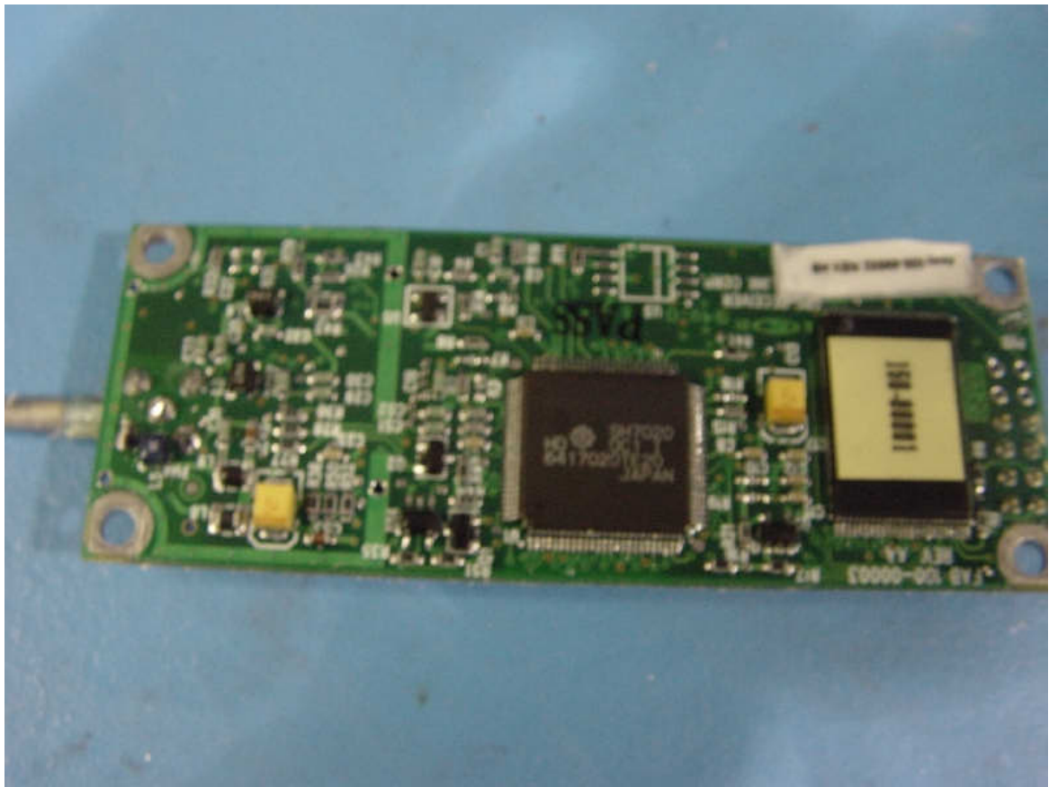
GPS module with RF shield removed (top)
