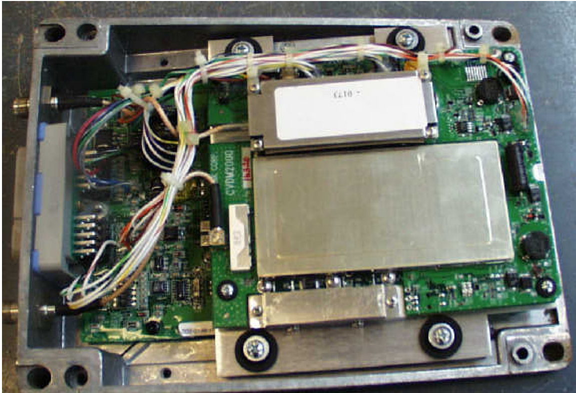
Deere ra with top half of enclosure removed showing Communications Interface PCB – view
