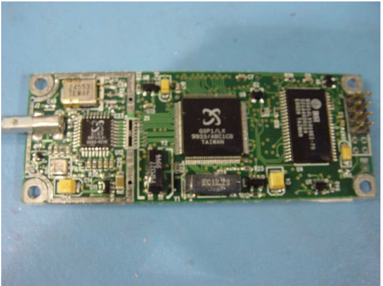
GPS module with RF shield removed (bottom)
