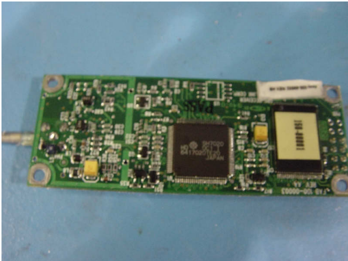
GPS module with RF shield removed (top)
