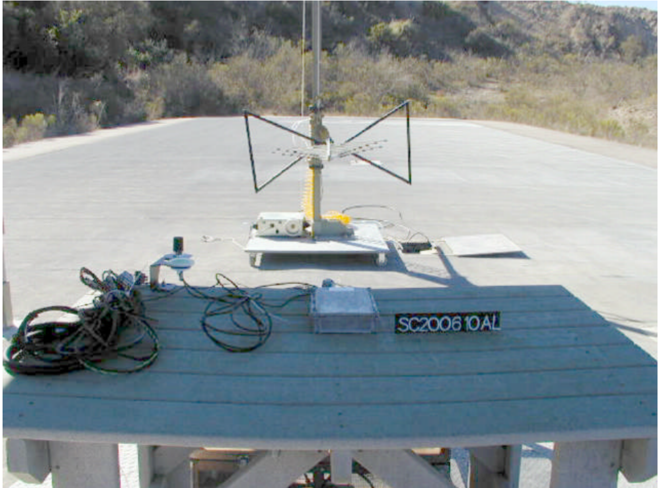
Photograph of Test Setup: Radiated Emissions
