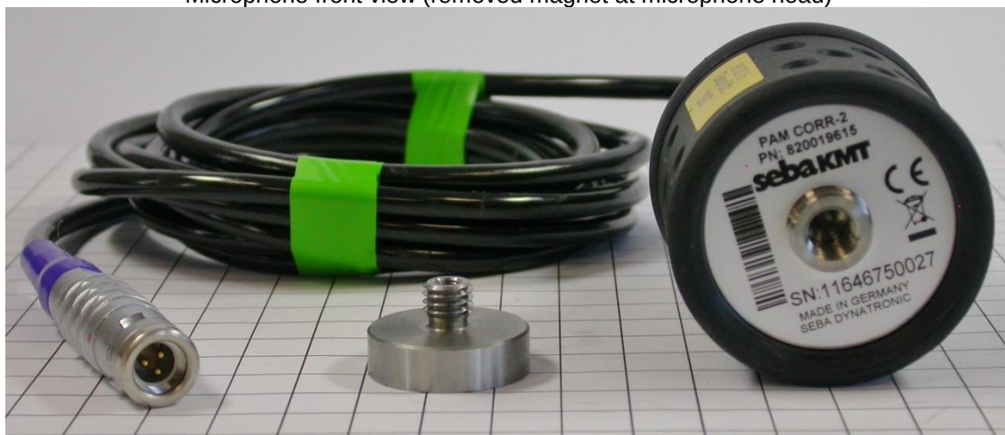
Microphone front view (removed magnet at microphone head)
