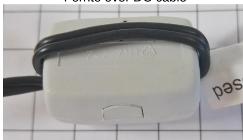
Ferrite over DC cable
