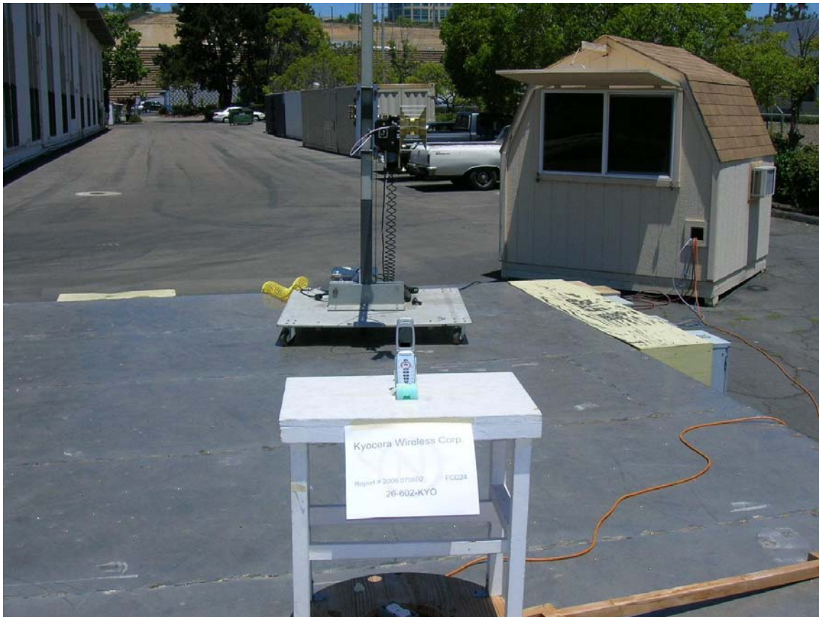
Figure 4. FCC, Part 24 Radiated Emissions Test Configuration
