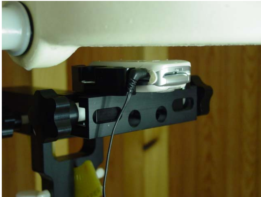
Body SAR setup with standard battery Closed (with 12mm air gap)
