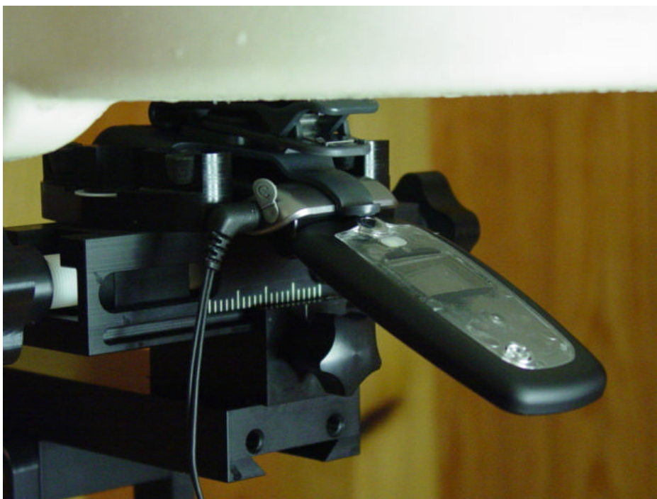
Figure 9E.8 body SAR setup Open (with Holster)
