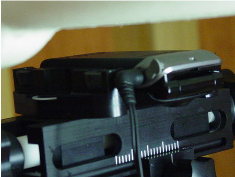
Figure 9E.3 body SAR setup closed (with 15mm air separation)
