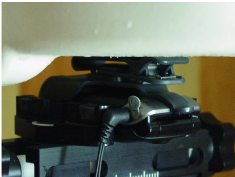
Figure 9E.7 body SAR setup Closed (with Holster)
