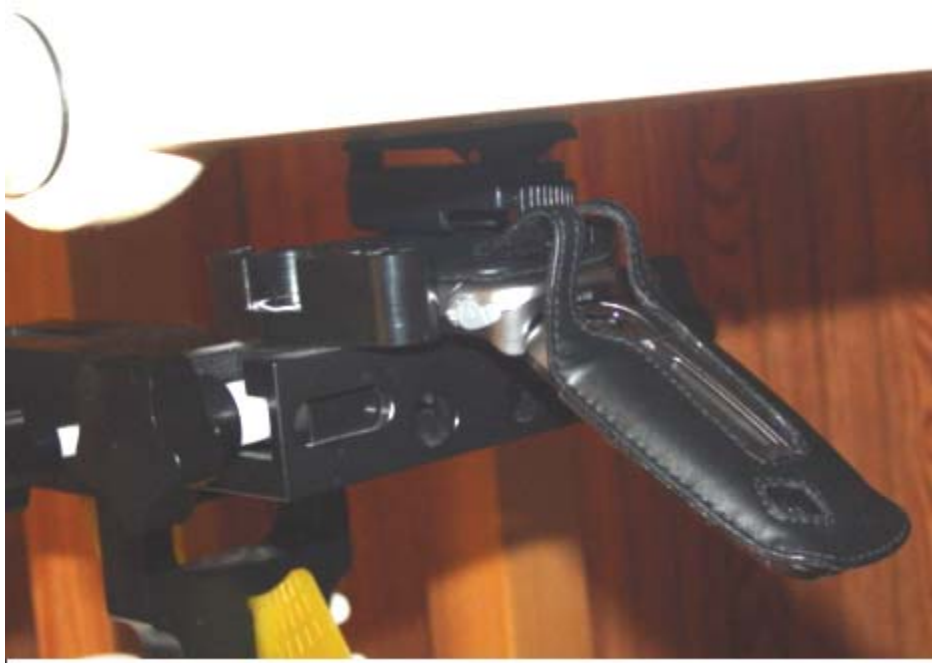
Figure 9. Body SAR setup open (with standard leather case)
