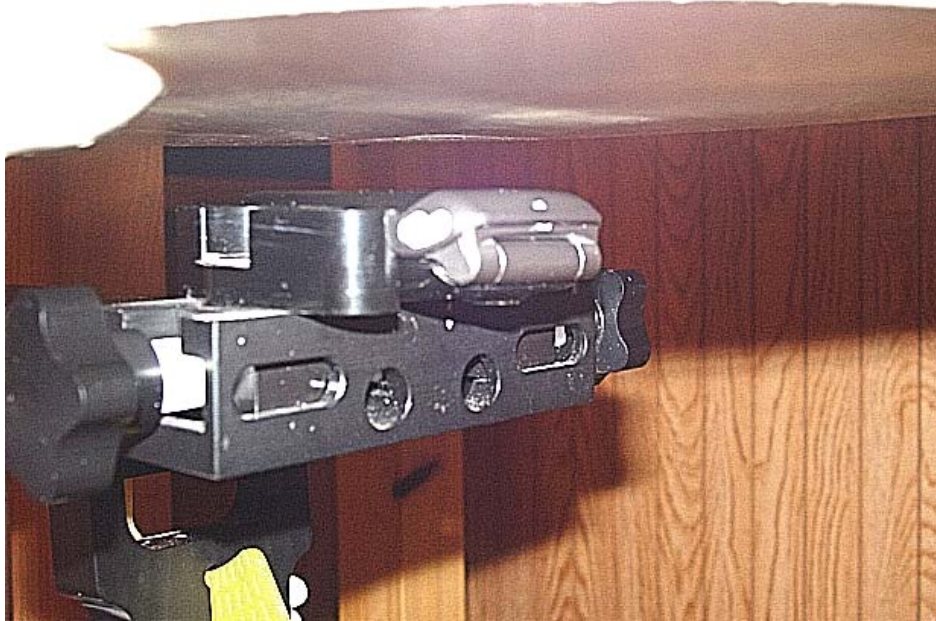
Figure 6. Body SAR setup closed (with 15mm air separation)
