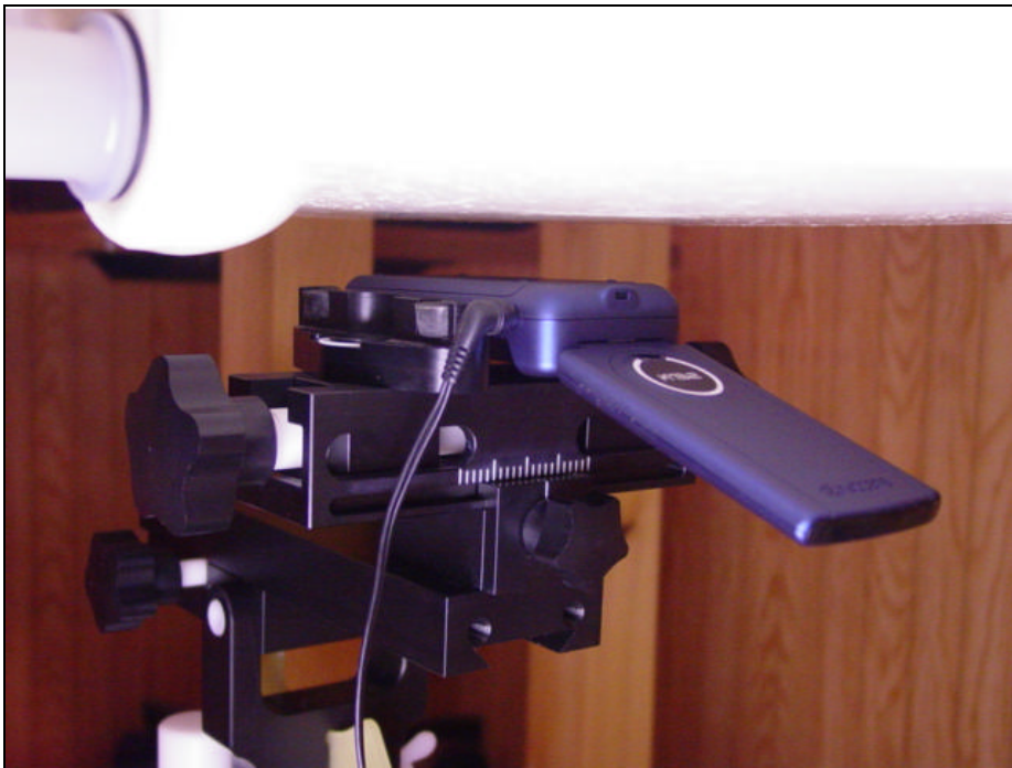
Figure 9E.4 body SAR setup open (with 15mm air separation)
