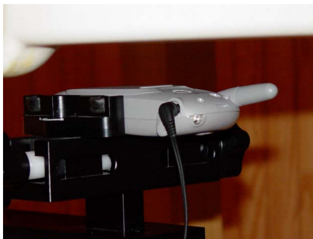
Figure 11.6 body SAR set-up (with 22.5mm air separation)
