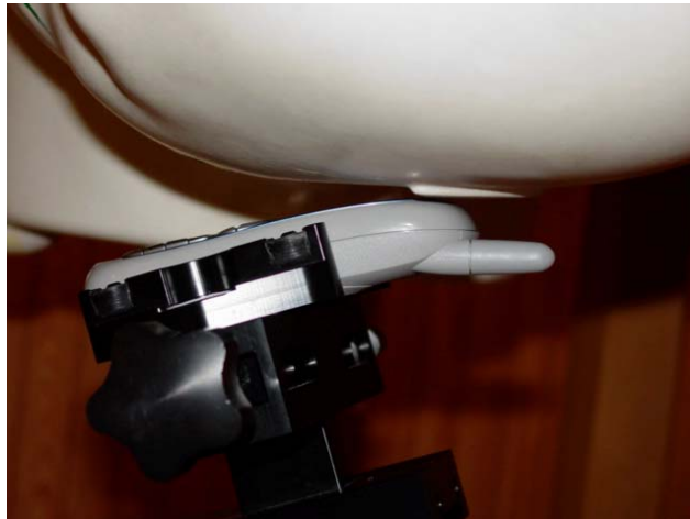
Figure 11.3 phone against the head (left tilt position)
