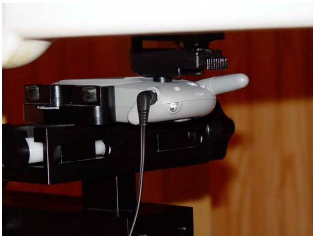
Figure 11.4 body SAR set-up (with belt clip)
