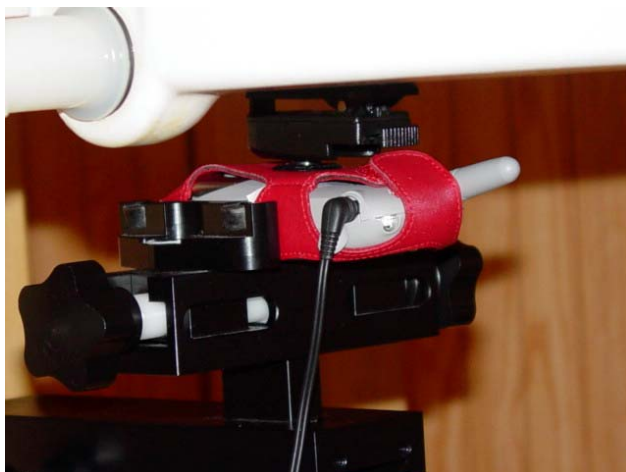
Figure 11.5 body SAR set-up (with leather case)
