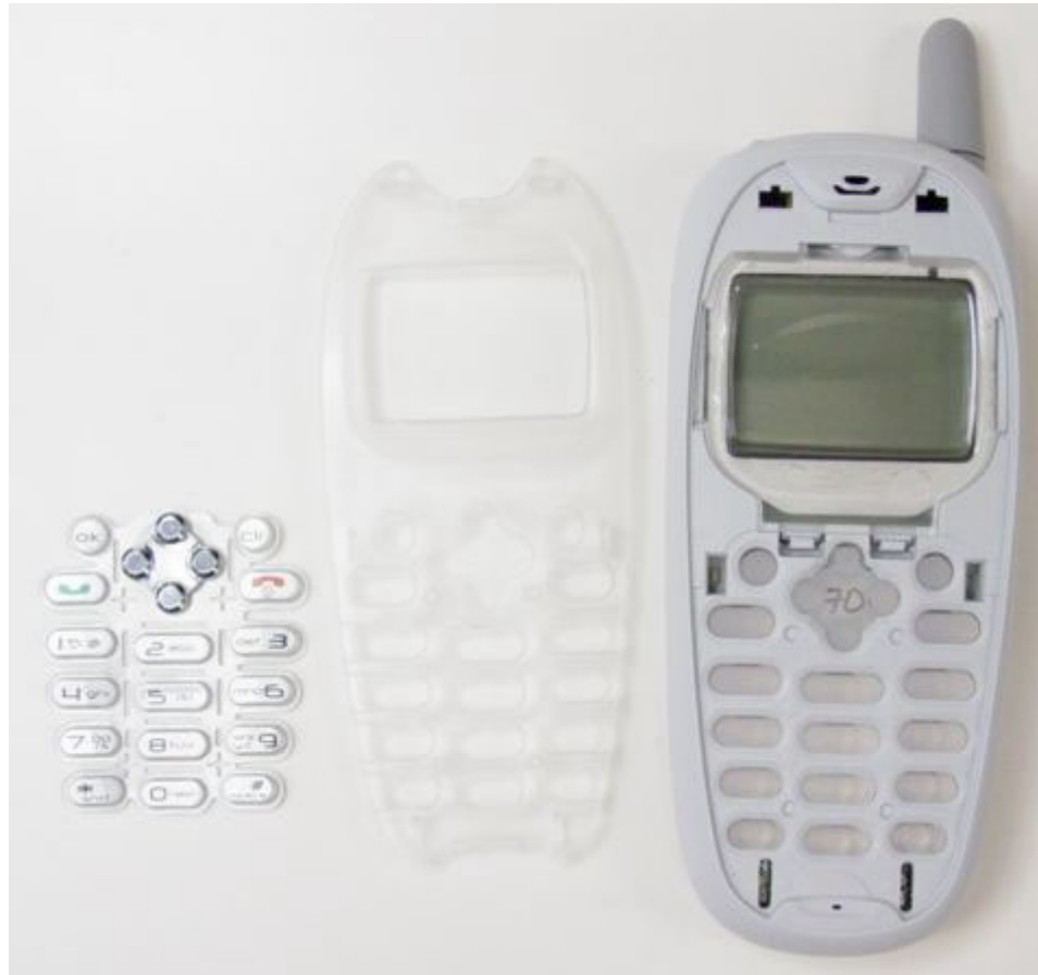
Front Housing with face plate off
