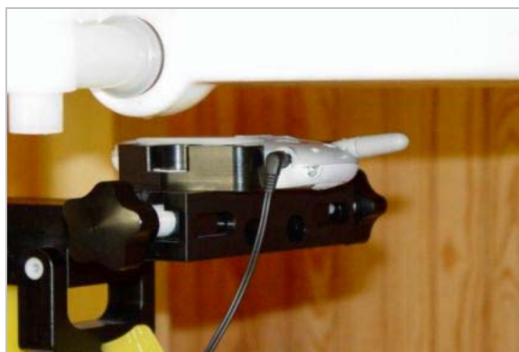
Figure 10.6 body SAR setup (with 22.5mm air separation)
