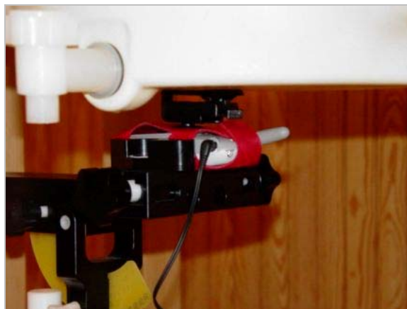
Figure 10.5 body SAR setup (with leather case)
