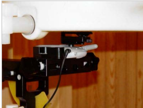
Figure 10.4 body SAR setup (with belt clip)
