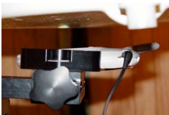
Figure 10.6 body sar setup (with 22.5mm air separation)
