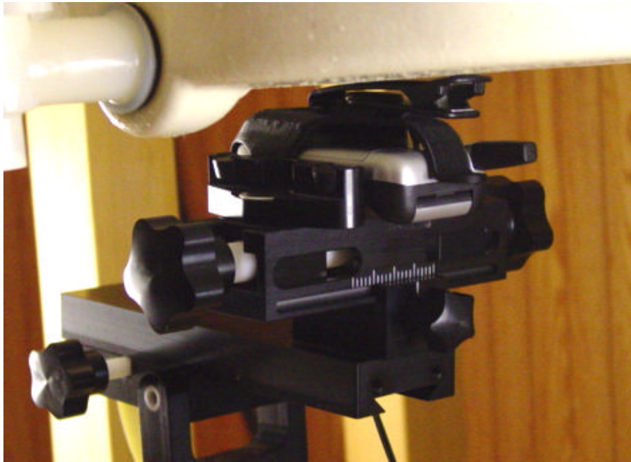
Figure 12.3 body SAR setup closed (with holster)
