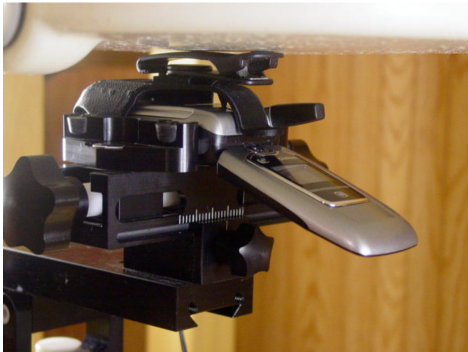
Figure 12.4 body SAR setup open (with holster)
