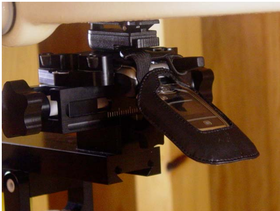
Figure 12.7 body SAR setup open (with leather case)
