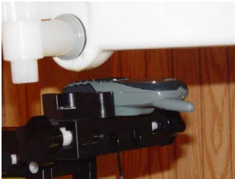
Figure 10.7 walkie-talkie radio setup (with 1 inch air separation)
