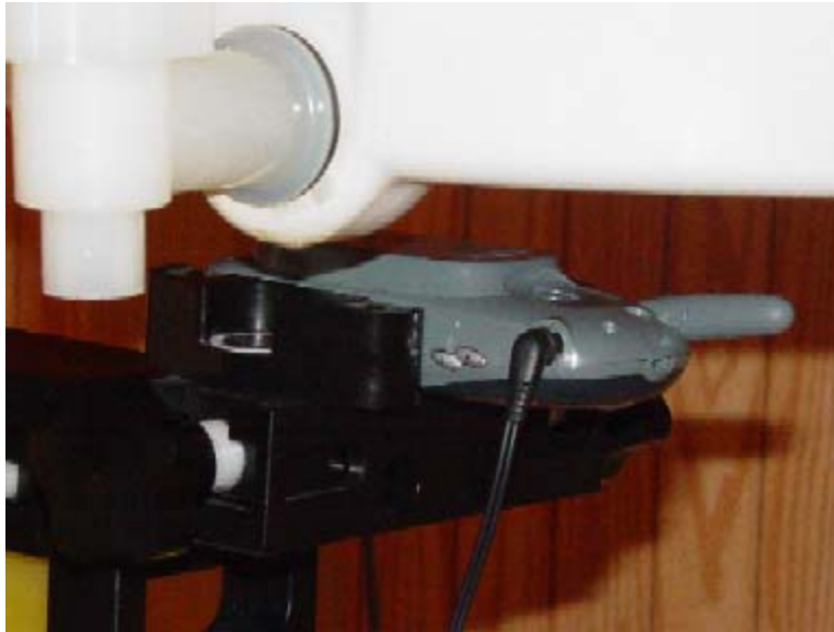
Figure 10.6 body SAR setup (with 25mm air separation)
