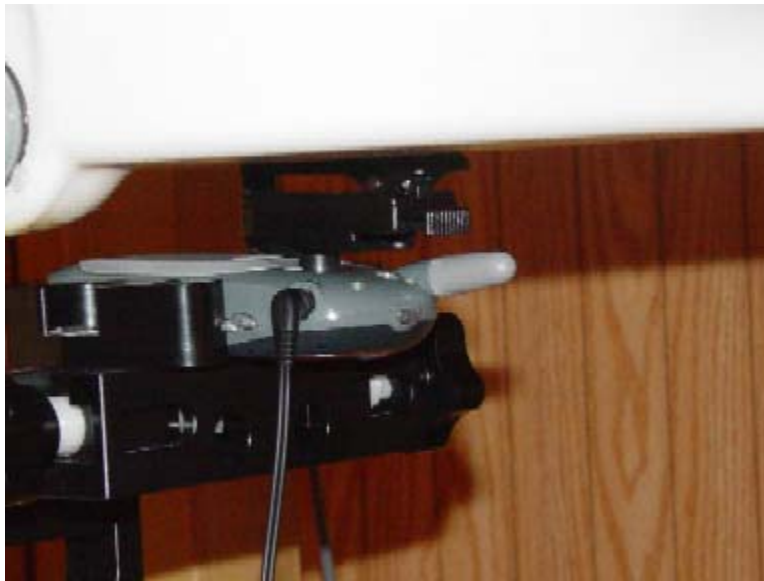
Figure 10.4 body SAR setup (with belt clip)
