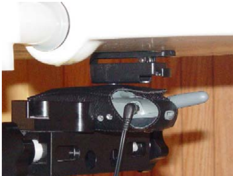
Figure 10.5 body SAR setup (with leather case)
