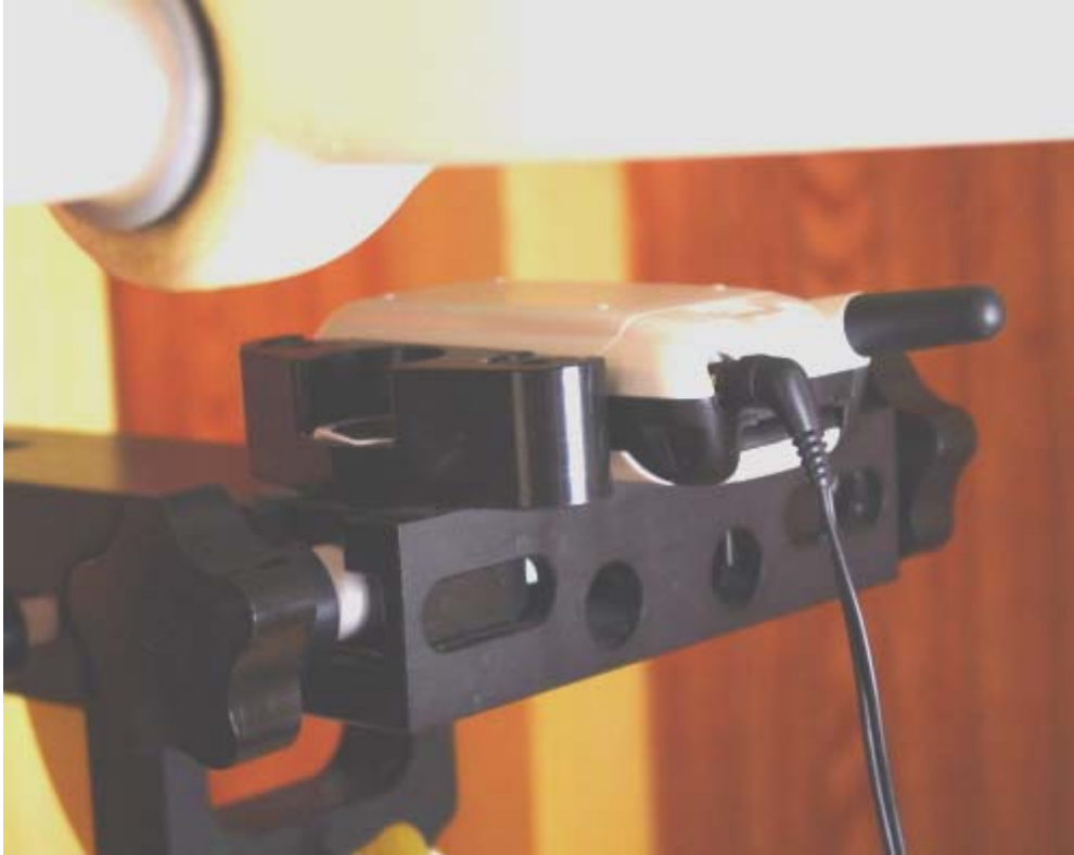
Figure 12.4 body SAR setup (with 22.5mm air separation)
