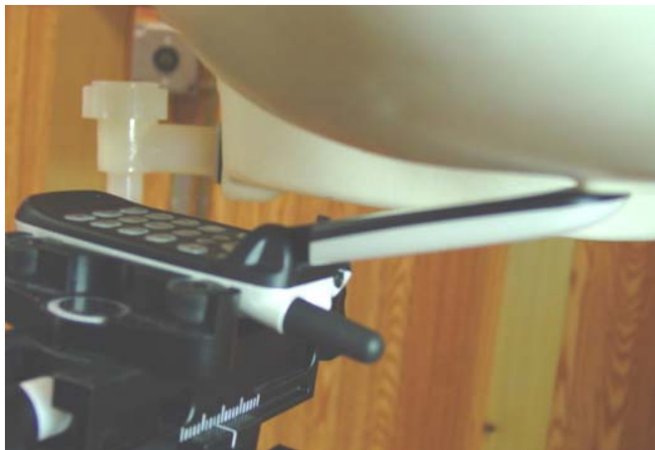
Figure 12.3 phone against the head (left tilt position)
