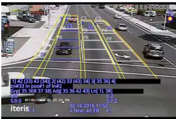
Good Lane Structure
