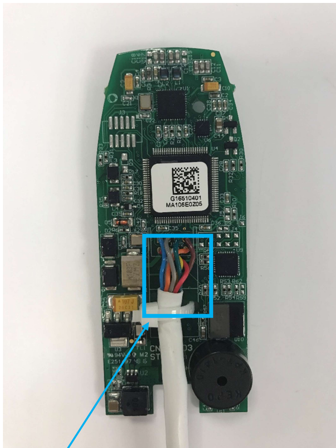
Cable directly plug on PCB
