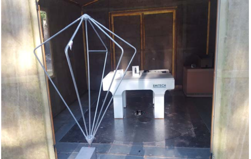
Radiated measurement on open area test site
