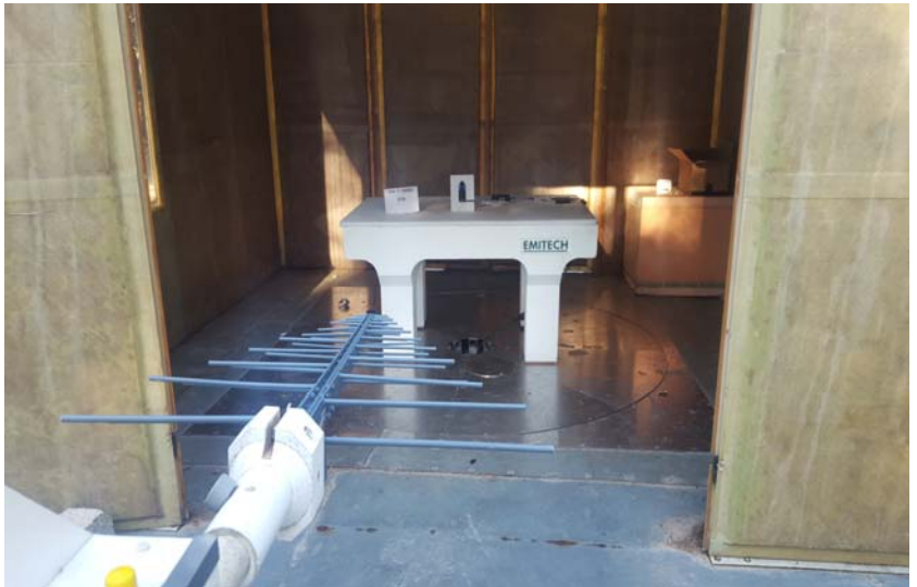
Radiated measurement on open area test site
